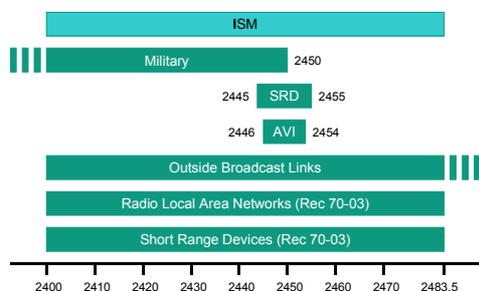
Notes: AVI - Automatic Vehicle Identification for railways. 500mW in 2446 - 2454 MHz.
