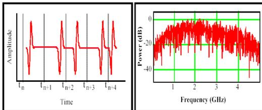
Pulse Position Modulated and Randomised Pulse Train and its Power Spectrum (taken from 'PulseOn Technology Overview', <http://www.timedomain.com>)
